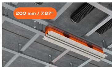
Minimum installation height: 200 mm / ≈ 7.87"
